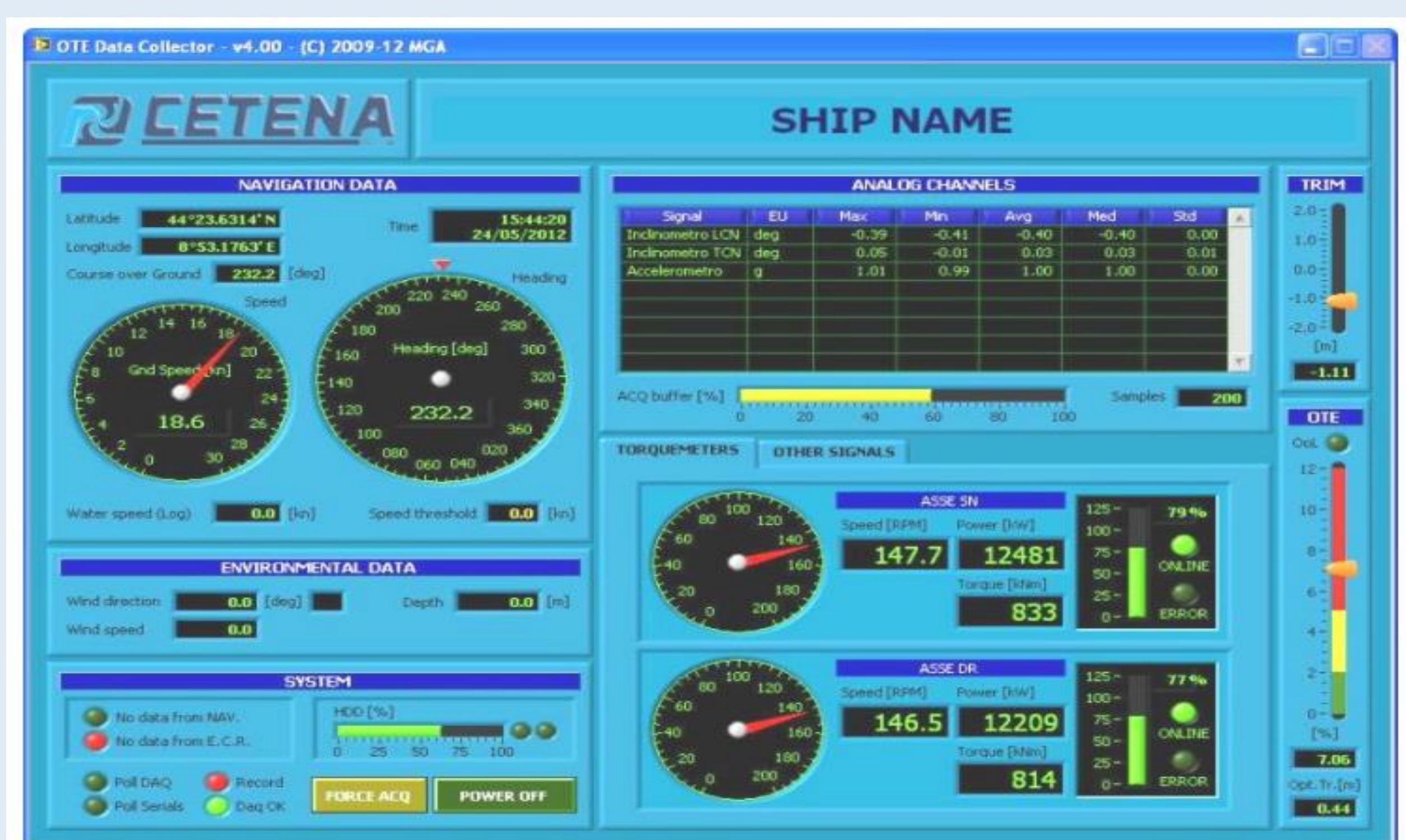
Long term monitoring system cockpit that will be installed on board
