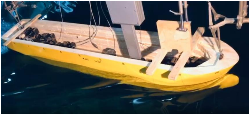
Loaded Condition (ITU, Ata Nutku Towing Tank)
