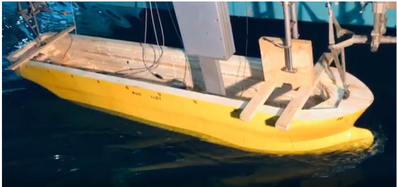
Ballast Condition (ITU, Ata Nutku Towing Tank)
