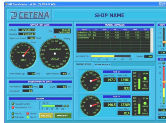
Long term monitoring system cockpit that will be installed on board
