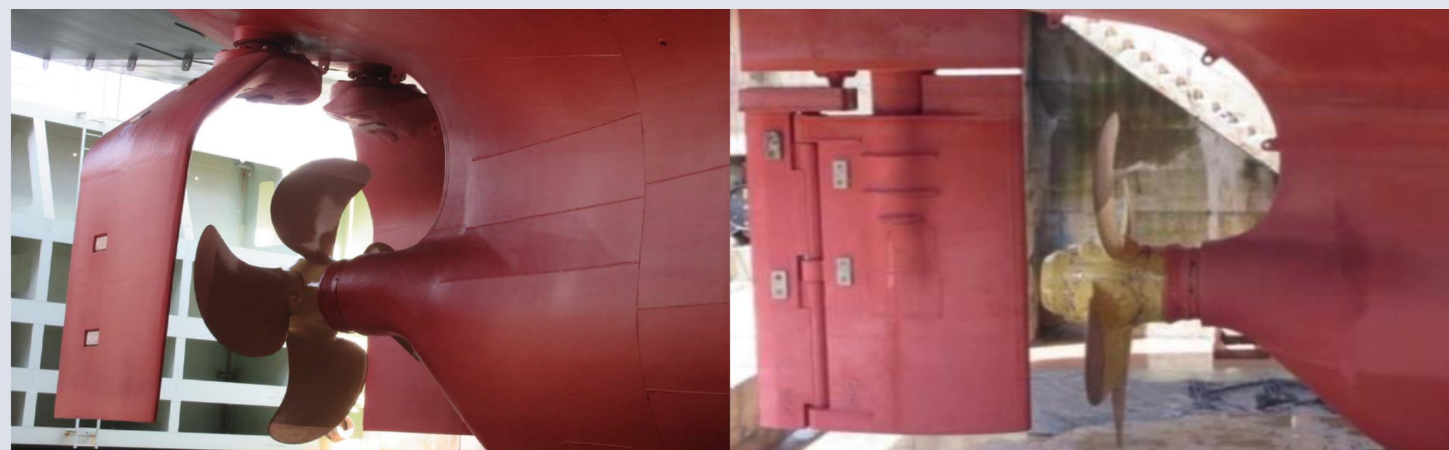
Figure 2: Retrofit GATE RUDDER and its counterpart conventional single rudder on Japanese twin container vessels
