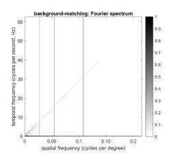
The left panel shows a horizontal slice through the stimulus and how that changes with time. The prey is visible as a diagonal stripe. The right panel shows the Fourier spectrum. The vertical lines in the right hand plot show the frequencies corresponding to the horizontal size of the prey (prey width = half a period, black line) and to the wide and narrow stripes (blue and red respectively).
