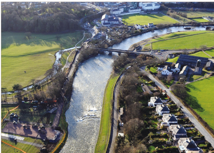
Figure 3. Aerial view looking downstream showing the collapsed Navvy or Navvies footbridge (top right), the damaged A596 Workington (Calva) bridge (centre) and the Barker Crossing site (bottom left)
